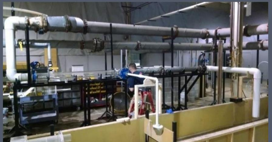
The 6" pipe test apparatus at the hydraulic lab.
