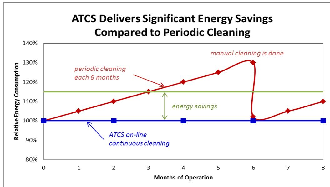
Figure 1. Continuous Tube Cleaning Technology Improves Chiller Efficiency
