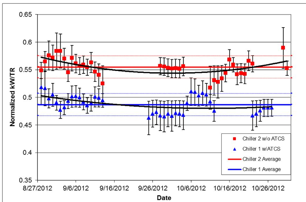
Figure 3. Chiller Energy Efficiency Improved 12% by Tube Cleaning Implementation <sup>5</sup>
