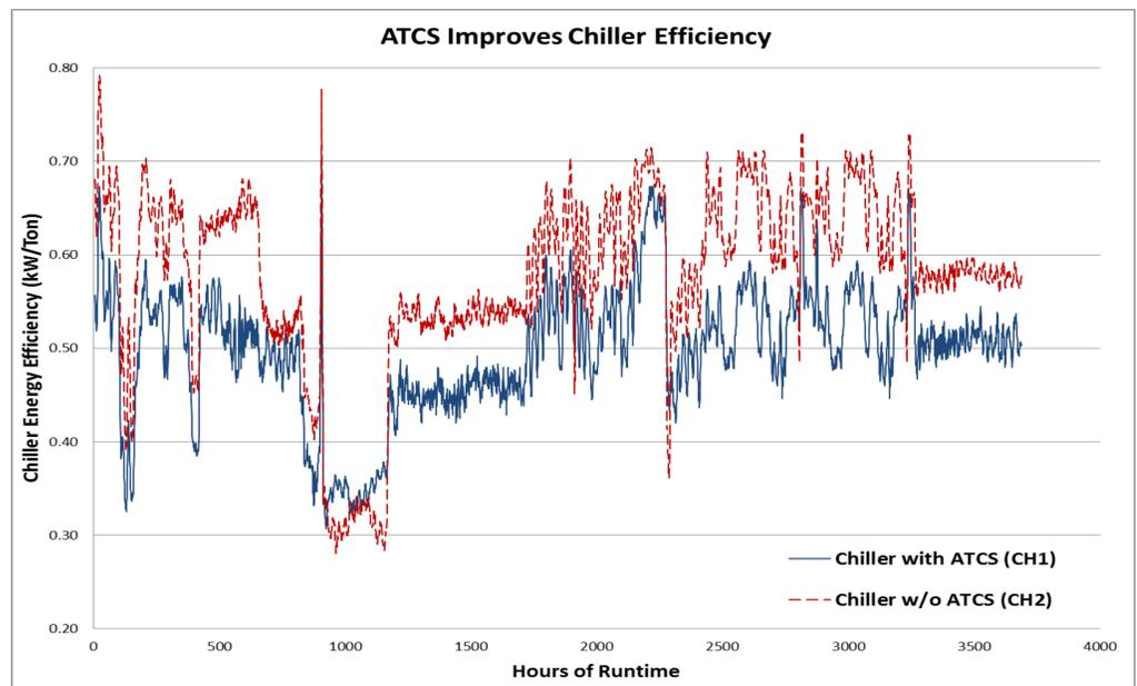
Figure 4. Tube Cleaning System Provides Continued Chiller Energy Efficiency Advantages
